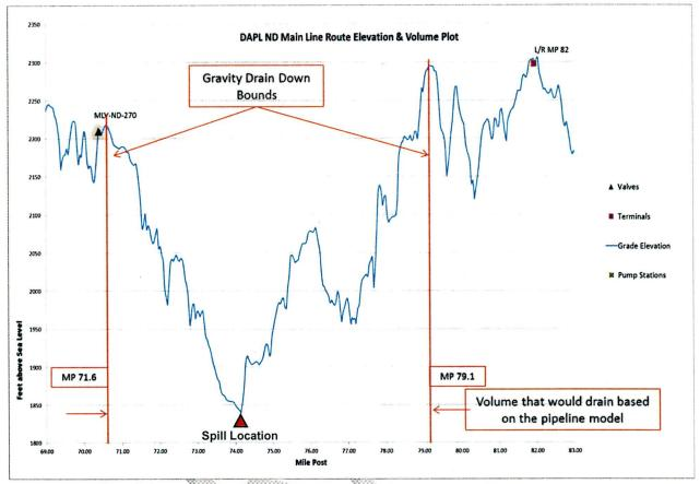
Worse-Case Scenario - Spill release based on the PHMSA model – Full-diameter opening with full pipeline drain down due to air purge.
